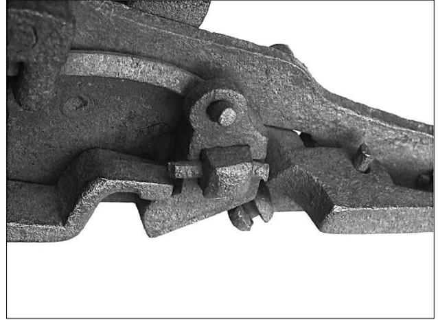
*The "push-rod" attached to the tumbler opens the pan-cover as the cock moves forward*
